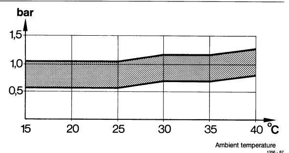
Low pressure in refrigerant circuit vs. ambient temperature
