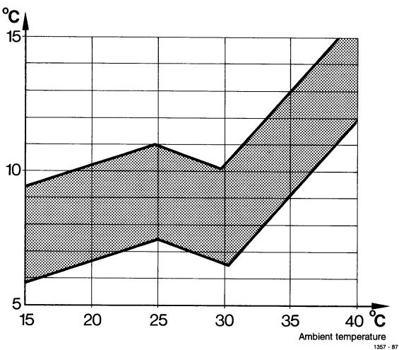
Air temperature at center nozzle vs. ambient temperature
