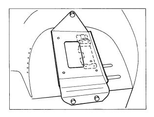
The holder is secured with 3 hexagon screws M 6 x 12.
