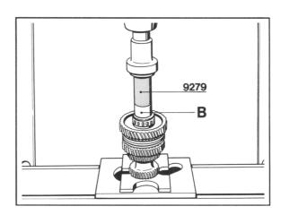
A = Special Tool 9279 B = Inner bearing race
