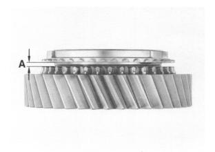
Preload gear block onto the shaft with 5 t. Use Special Tool 9279 for this.
