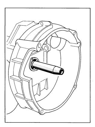
2. Fill the area between sealing lips with grease (e.g. Olista Longtime 3 EP)
