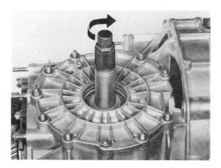
Turn measuring mandrel carefully until the dial-gauge extension is vertical to the facing edge of the drive-pinion head. At this point, the pointer of the dial gauge reaches max. deflection (reverse point), and the dial gauge must be read.
