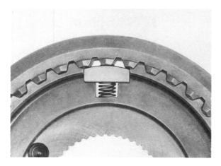
Installation position of gearshift sleeve. The dotting mark must be fitted centrally in relation to the driver dogs.
