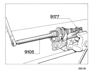
Use a suitable tool (e.g. Kukko 17 - 1) to press all parts off the input shaft over the 2nd gear wheel.
