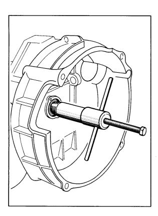
4. Pull out seal by screwing in the hexagon head screw.
