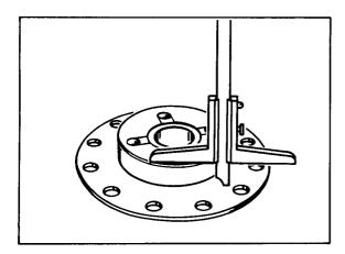
Calculate clearance "c" inside casing.
