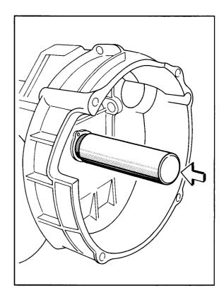
4. Install guide tube and tighten fastening screws with 10 Nm (7.5 ft.lb.)
