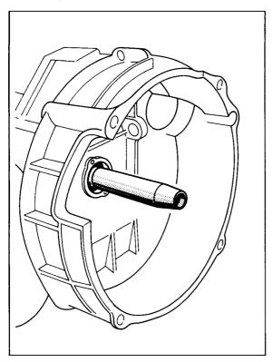
3. Use Special Tool **9256** to drive the oil into place.
