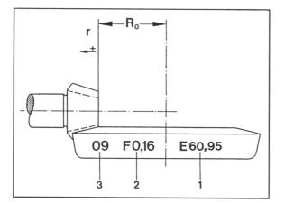
Set adjusting ring of measuring mandrel VW 385/1 to dimension "a".
