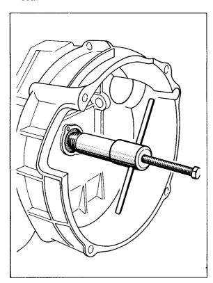
4. Screw in the hex bolt and pull out oil seal.
