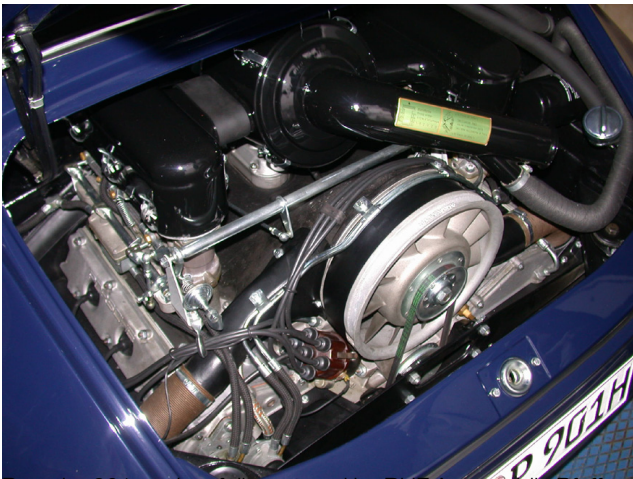
Porsche 901 engine, fully restored by RUF Automobile Pfaffenhausen Germany. Photo: Adrian Streater
